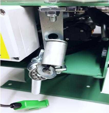
For safety reasons your clay pigeon trap is supplied with the main spring detached. Remove the cable ties carefully to access the parts.
