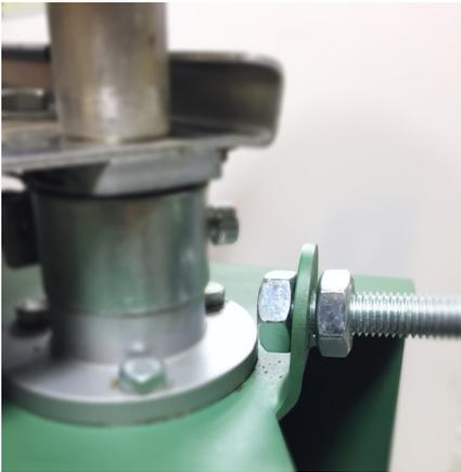
Screw the 10mm studding into the front of the steel body and lock off with the 10mm nut
