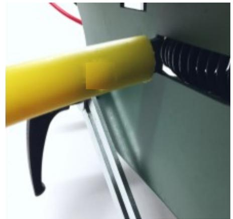
Push the ends of the safety rings onto the steel mounts on each side of the trap to secure.
