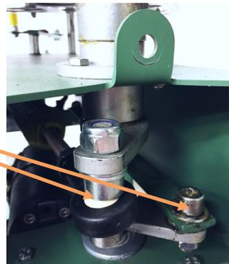
Lubricate these areas. Avoid putting any grease onto the plate of the throwing arm.
